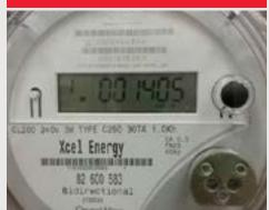
This meter can be programmed for several rate options including PV Time of Use. The Bridge Meter Statement is similar to the Standard Net Meter Statement above.
