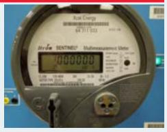
This is a standard meter that determines how many kWh your solar system is producing each month. If you are participating in the Solar\*Rewards program then your production meter will also be used to calculate your monthly Renewable Energy Credits (RECs) payments. The Production meter has a separate account number. The monthly statements are sent to the owner of the PV system.
